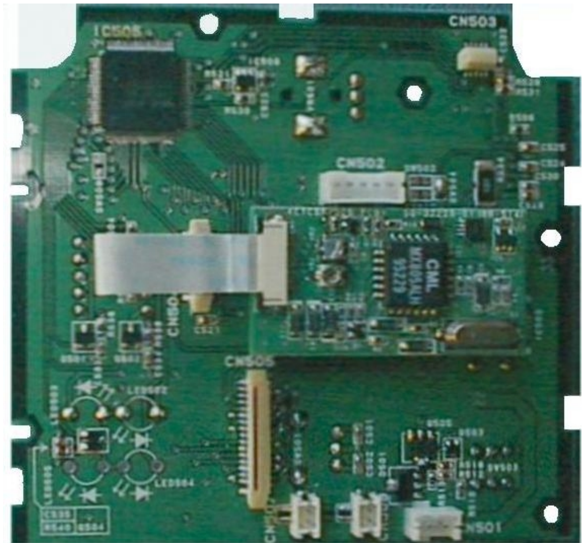
Fig. 3 Disp/Cont PCB rear – with CTSS/DCS PCB mounted.
