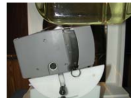
Figure 14.2 Body SAR Test Setup
