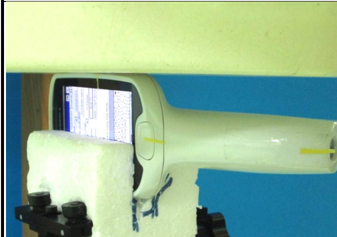
Hand-held Mode, ANT Side of EUT with 0 cm Gap
