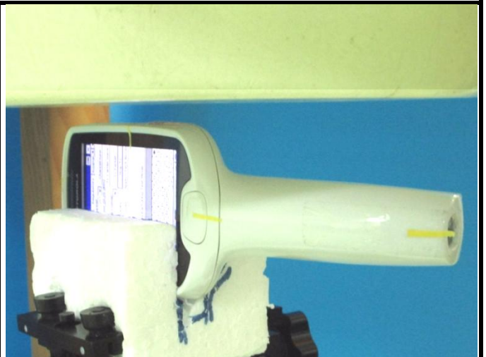
Body-worn Mode, ANT Side of EUT with 1.0 cm Gap
