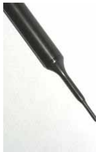
Fig. 5.2 EX3DV3 E-field Probe
