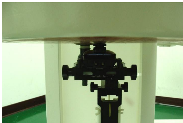
Face of the DUT with Battery 1 + Scanner 2 + Keypad 2 (Holster 1 with Phantom 0 cm Gap)
