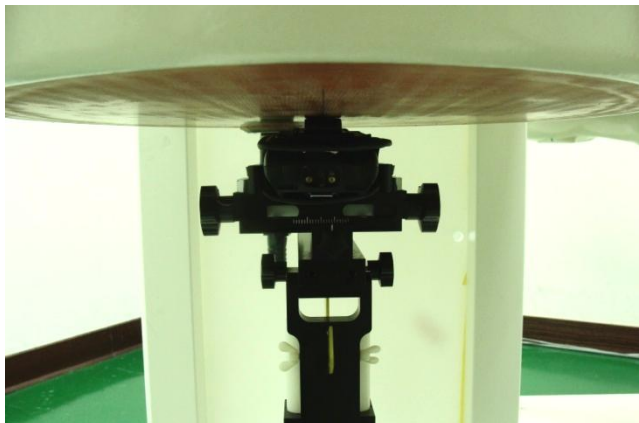
Face of the DUT with Battery 1 + Scanner 2 + Keypad 2 (Holster 2 with Phantom 0 cm Gap)
