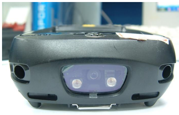
DUT with Scanner 2 (SE4500 Scanner)
