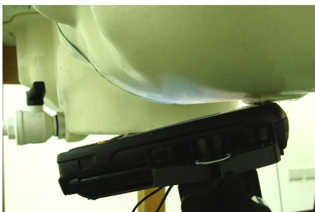
Left Tilted - DUT with Battery 2 + Scanner 2 + Keypad 3
