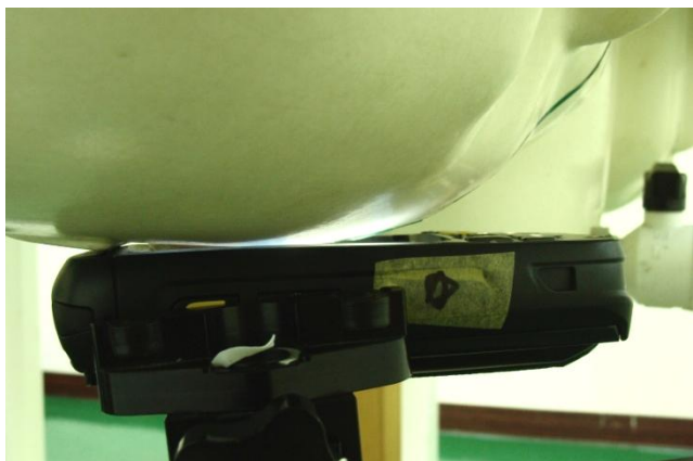
Right Cheek - DUT with Battery 2 + Scanner 1 + Keypad 1
