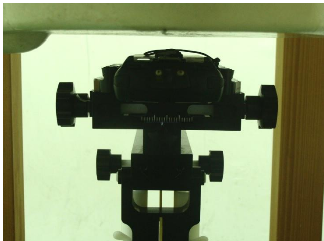
Bottom of the DUT with Battery 1 + Scanner 2 + Keypad 1 (with Phantom 1.5 cm Gap)
