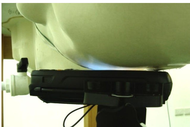
Left Cheek - DUT with Battery 2 + Scanner 2 + Keypad 3
