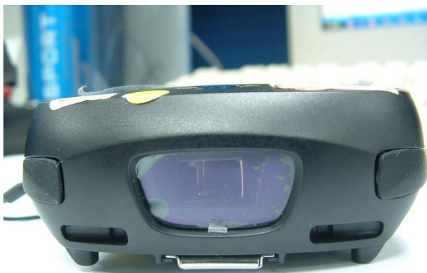
DUT with Scanner 1 (SE960 Scanner)
