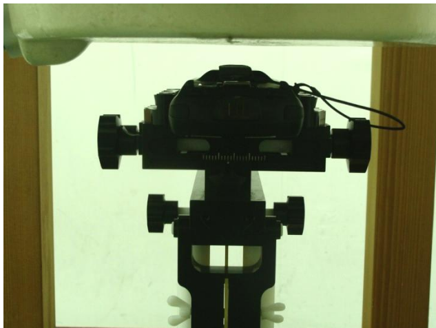
Bottom of the DUT with Battery 2 + Scanner 1 + Keypad 1 (with Phantom 1.5 cm Gap)
