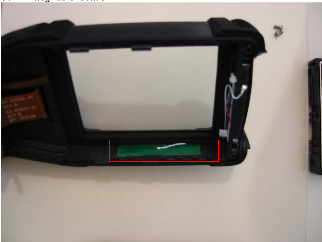
802.11 abg antenna locations (both sides of front display)
