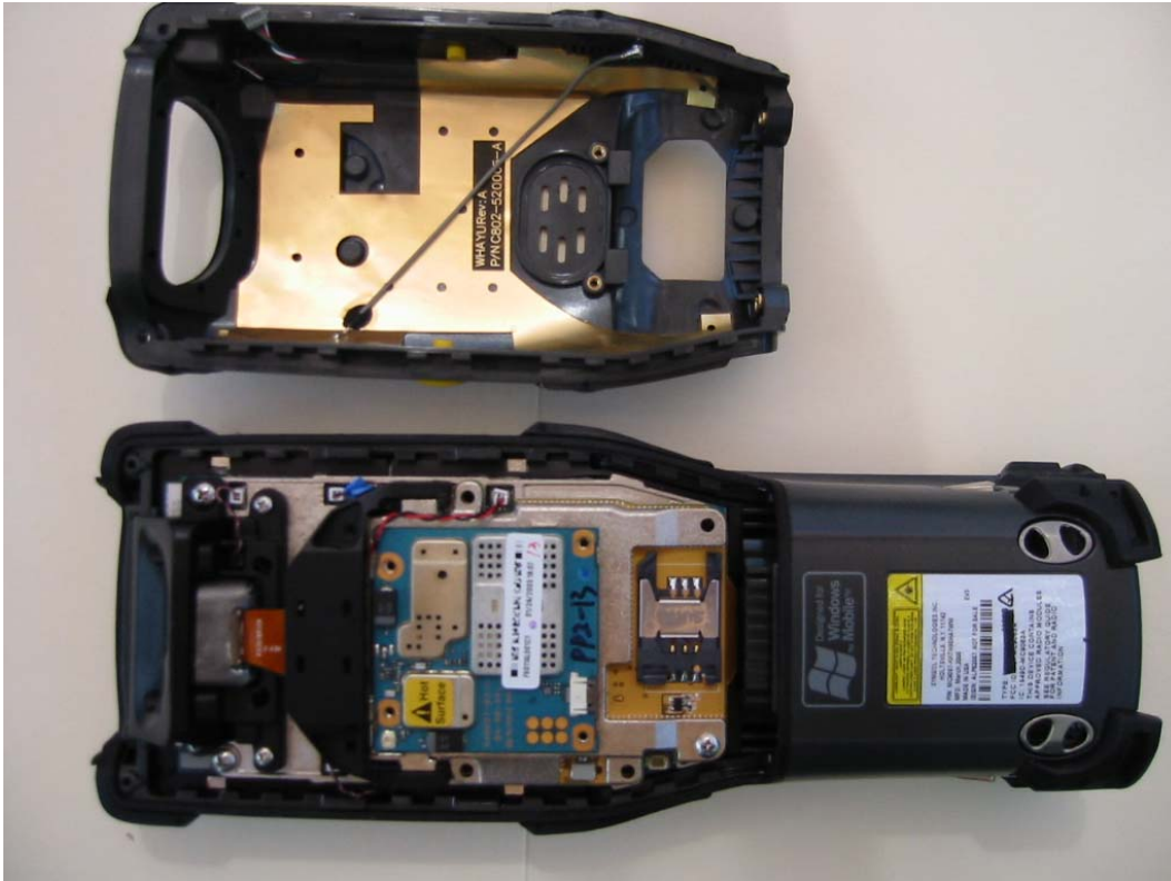
IDEN antenna inside back housing (shown opened above terminal)
