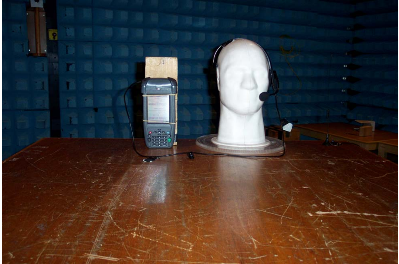
Radiated Emissions Set Up
