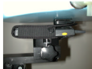
Figure 17. Body SAR Test Setup
