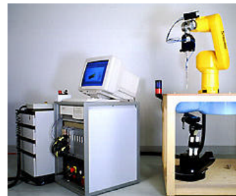
Fig. 1 SAR Test Setup
