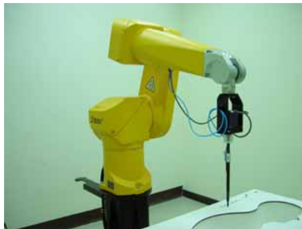
Fig. 5.2 Probe setup on robot
