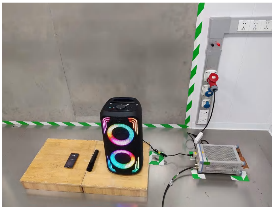
Photograph 3: Set-up photo for Conducted Emission on AC Mains
