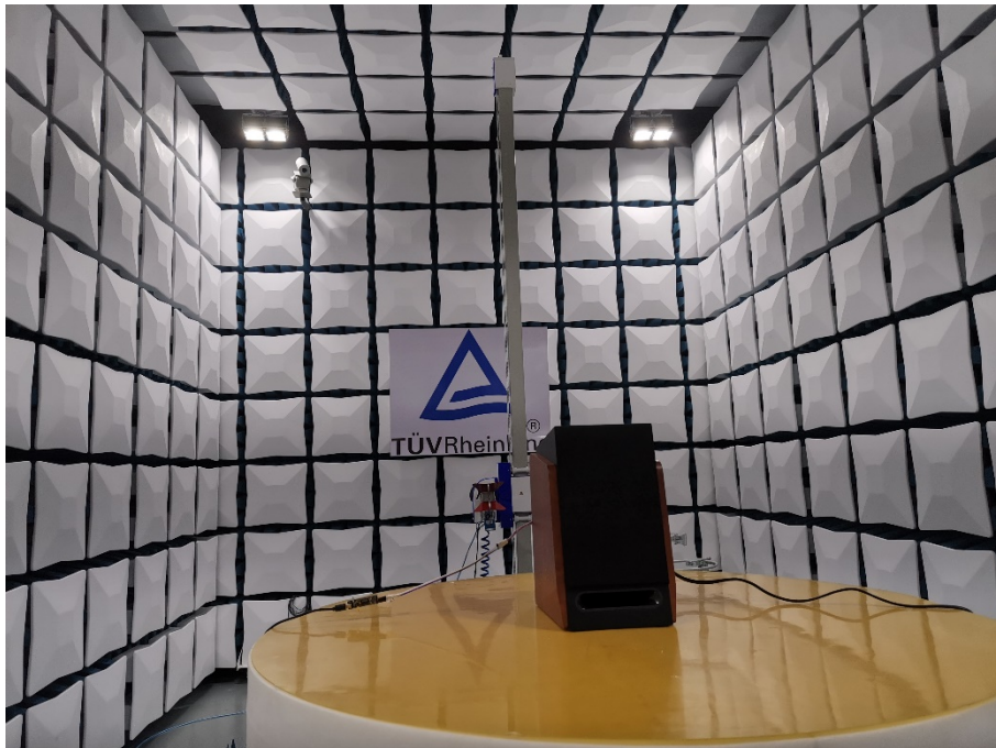
Photograph 2: Set-up for Radiated Spurious Emission, Above 1GHz
