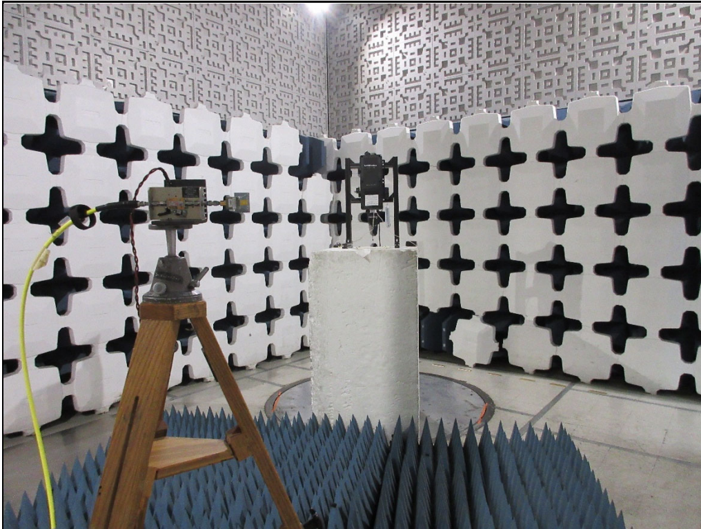
Test Setup for Spurious Radiated Emissions, Above 18GHz – Antenna Polarization Horizontal
