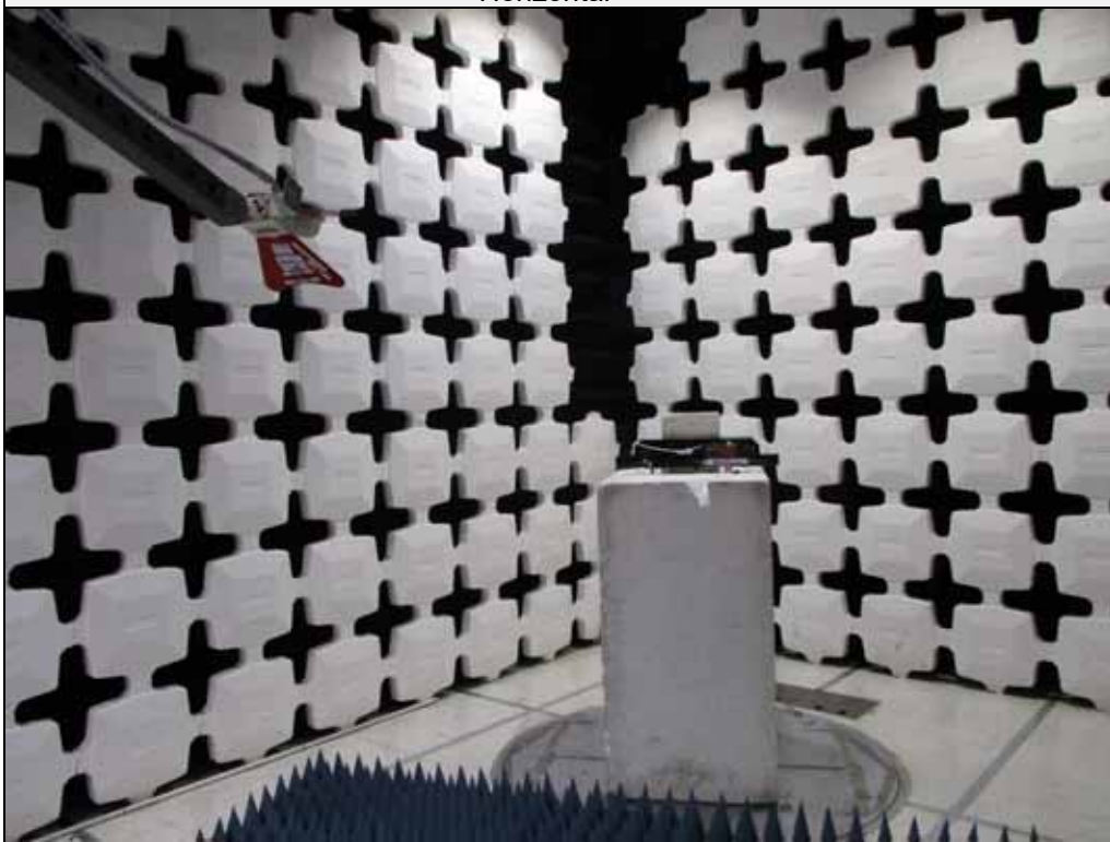
Test Setup for Spurious Radiated Emissions, Above 1GHz – Antenna Polarization Vertical
