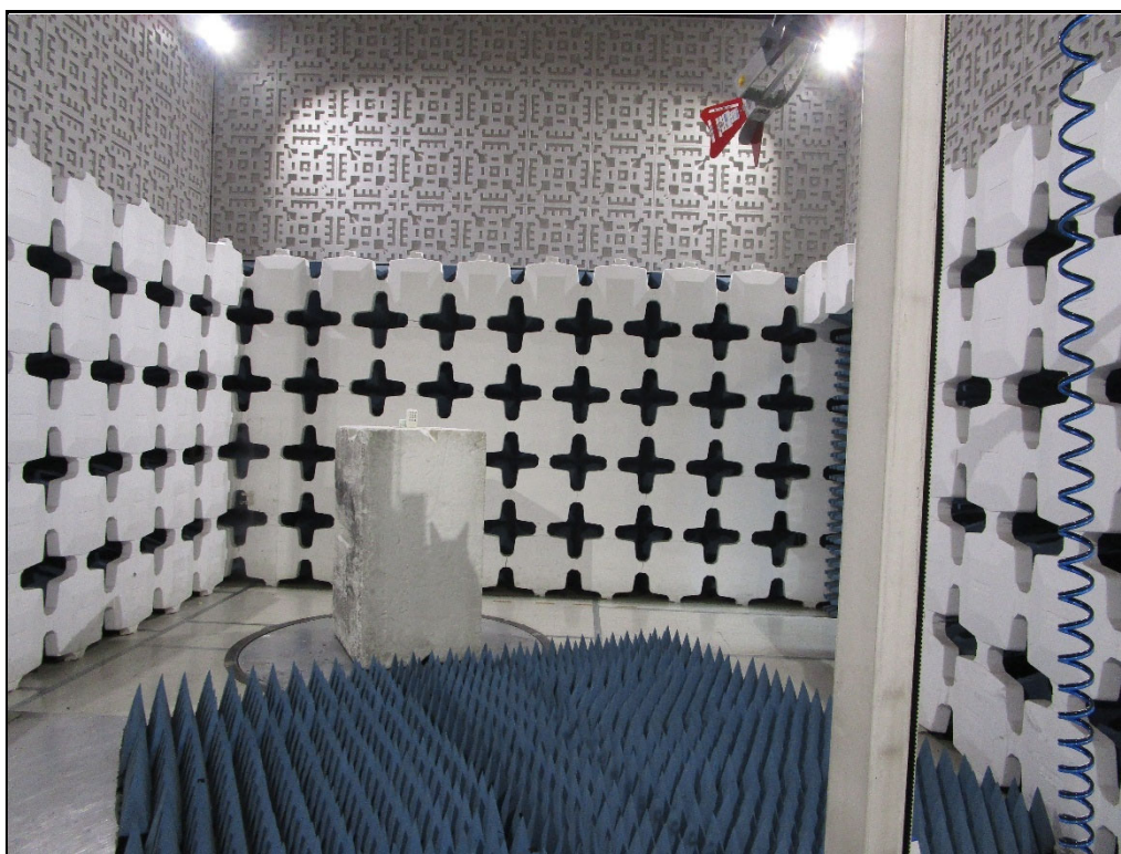
Test Setup for Spurious Radiated Emissions, 1 – 18GHz – Antenna Polarization Horizontal
