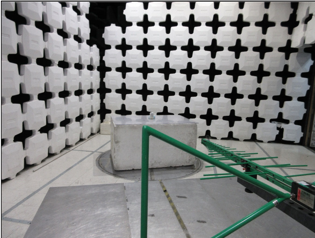
Test Setup for Spurious Radiated Emissions, 30MHz – 1GHz – Antenna Polarization Horizontal
