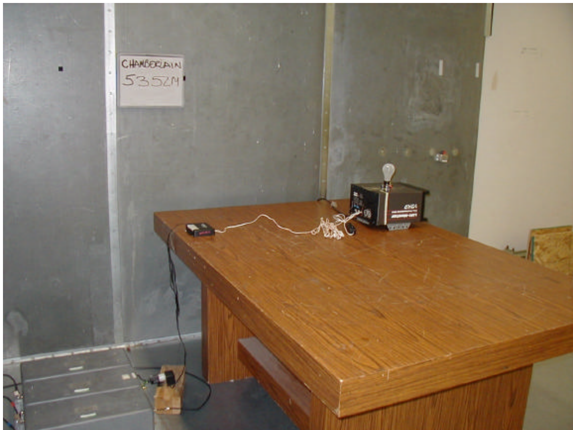
Conducted Voltage Test Setup Photos of - 535-315LM
