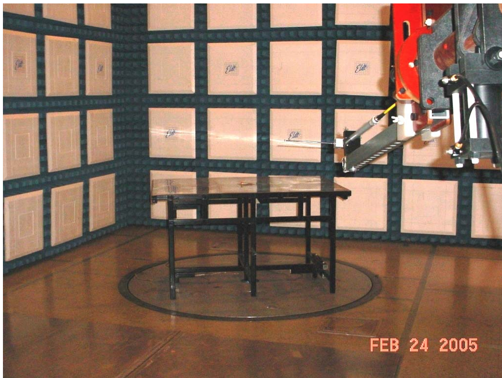
Test Setup for Radiated Emissions Horizontal Polarity
