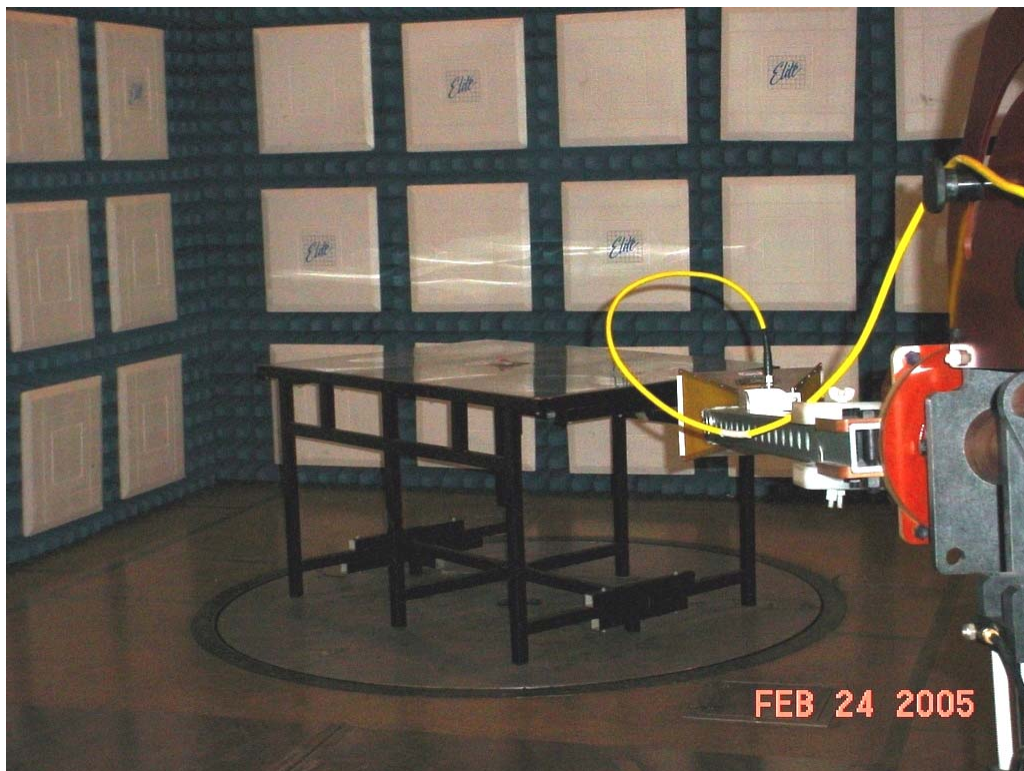
Test Setup for Radiated Emissions Vertical Polarity
