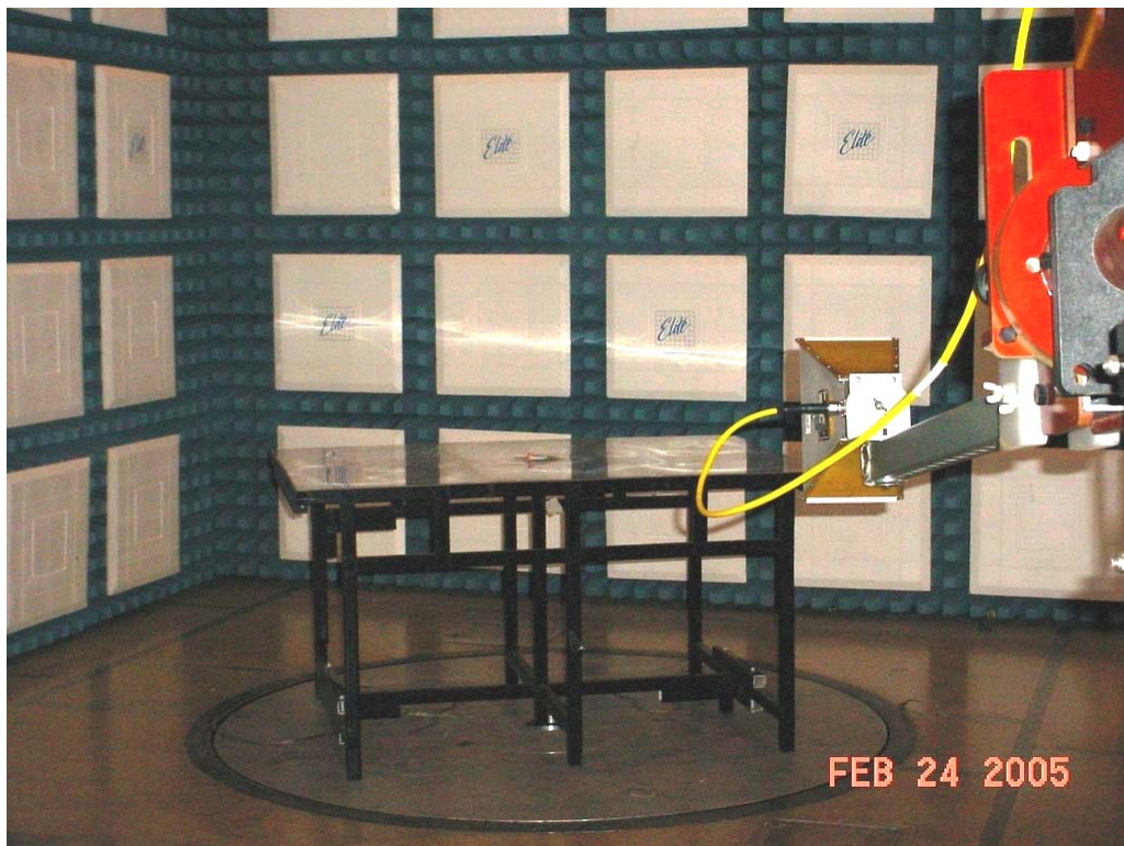
Test Setup for Radiated Emissions Horizontal Polarity
