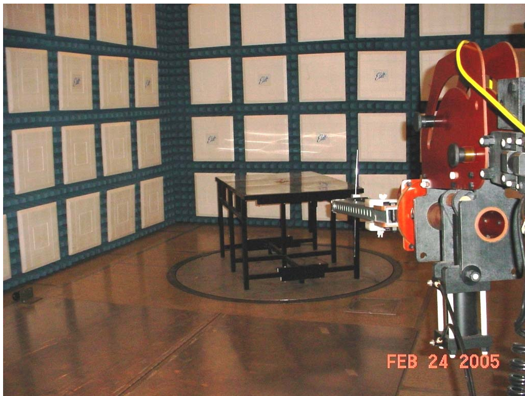
Test Setup for Radiated Emissions Vertical Polarity
