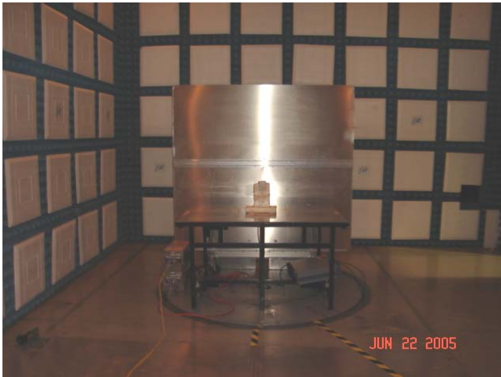
Test Set-up for Conducted Emissions
