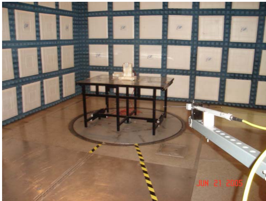
Test Set-up for Radiated Emissions Horizontal Polarity
