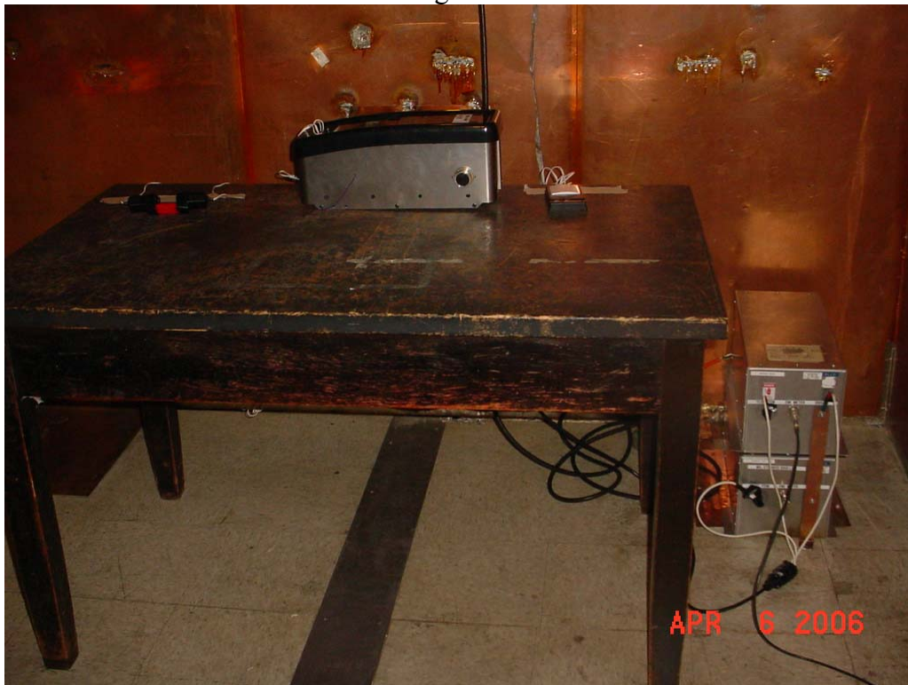
Test Set-up for Conducted Emissions
