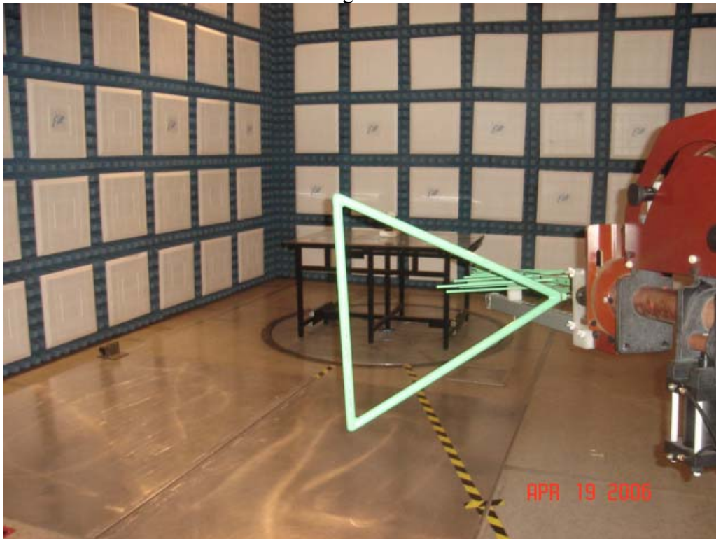
Test Set-up for Radiated Emissions – Horizontal Polarization
