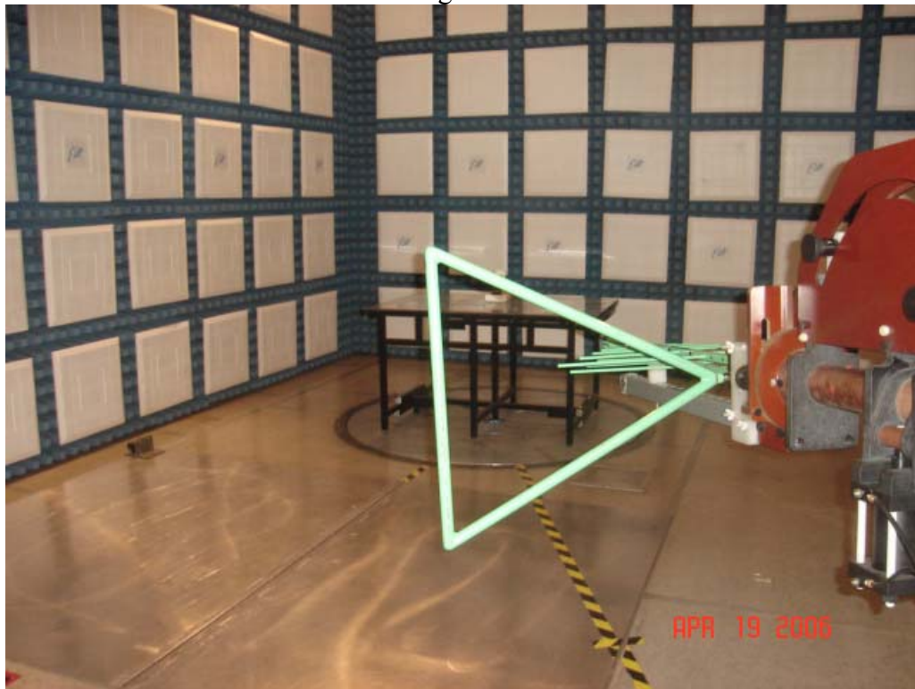
Test Set-up for Radiated Emissions – Horizontal Polarization
