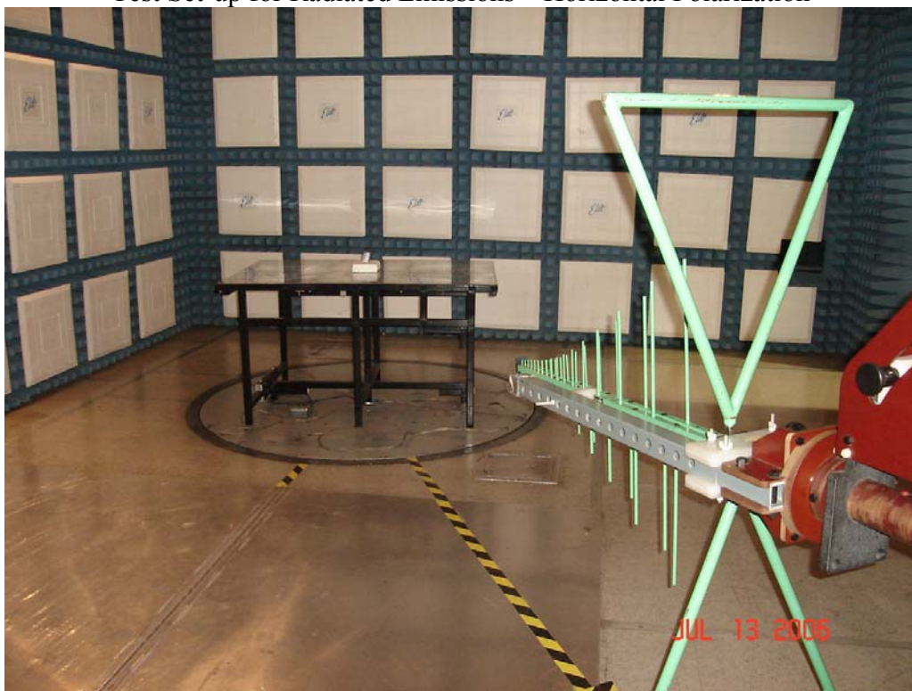
Test Set-up for Radiated Emissions – Horizontal Polarization
