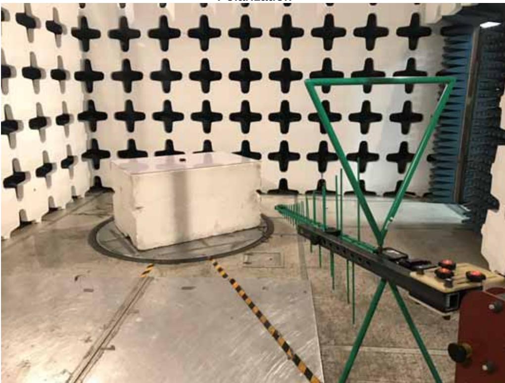
Figure 3 - Test Setup for Radiated Emissions, 30MHz to 1GHz – Vertical Polarization
