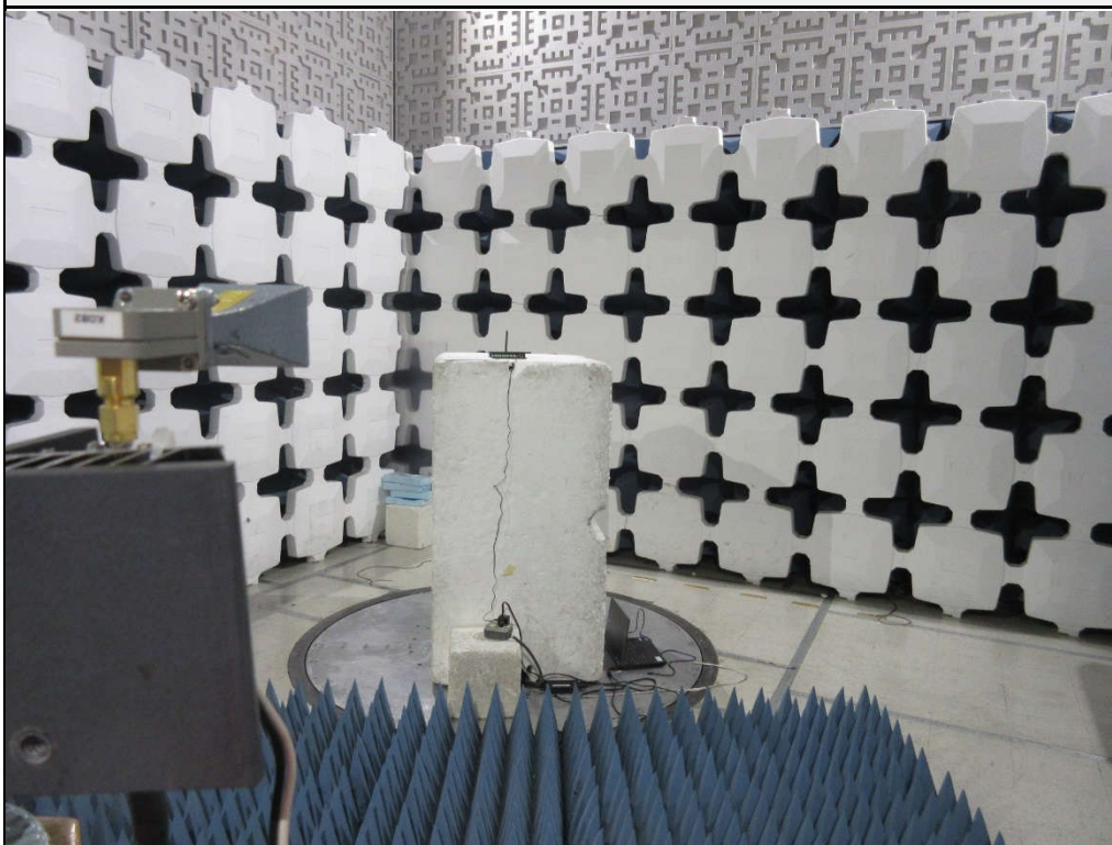
Test Setup for Spurious Radiated Emissions, 18 – 25GHz – Antenna Polarization Vertical
