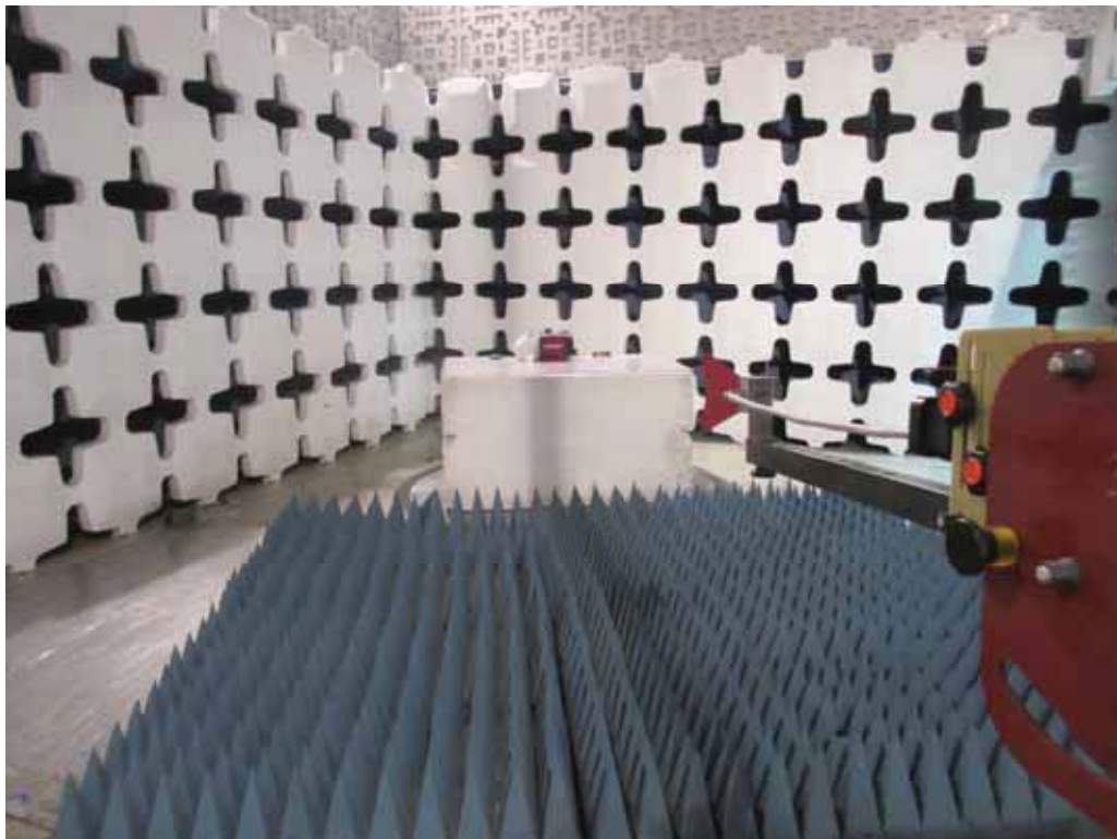
Test Setup for Radiated Emissions (Receiver) – 1 to 10GHz, Vertical Polarization
