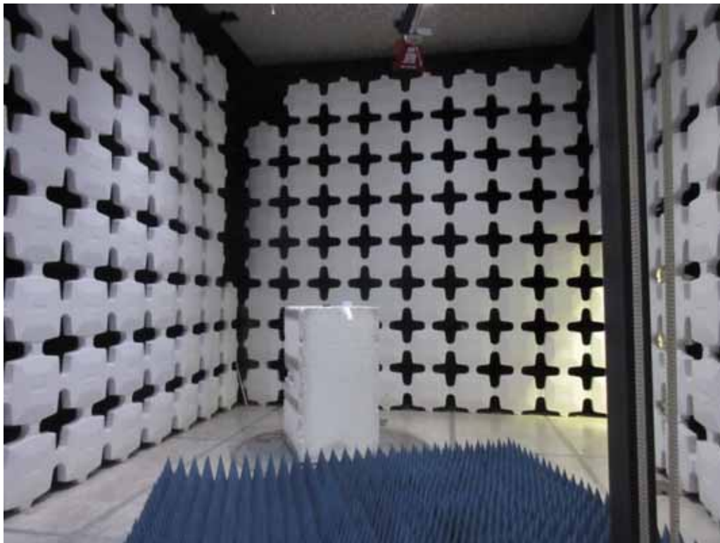
Test Setup for Radiated Emissions, 1 to 4GHz – Vertical Polarization
