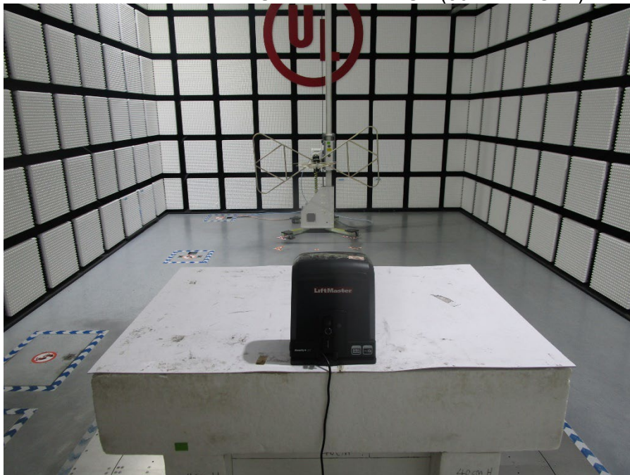
RADIATED RF MEASUREMENT SETUP (30MHz~1GHz)
