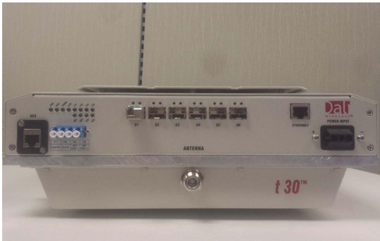
t30 800 PS Connector Panel View
