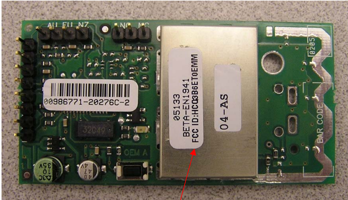
PCB with FCC ID number identification
