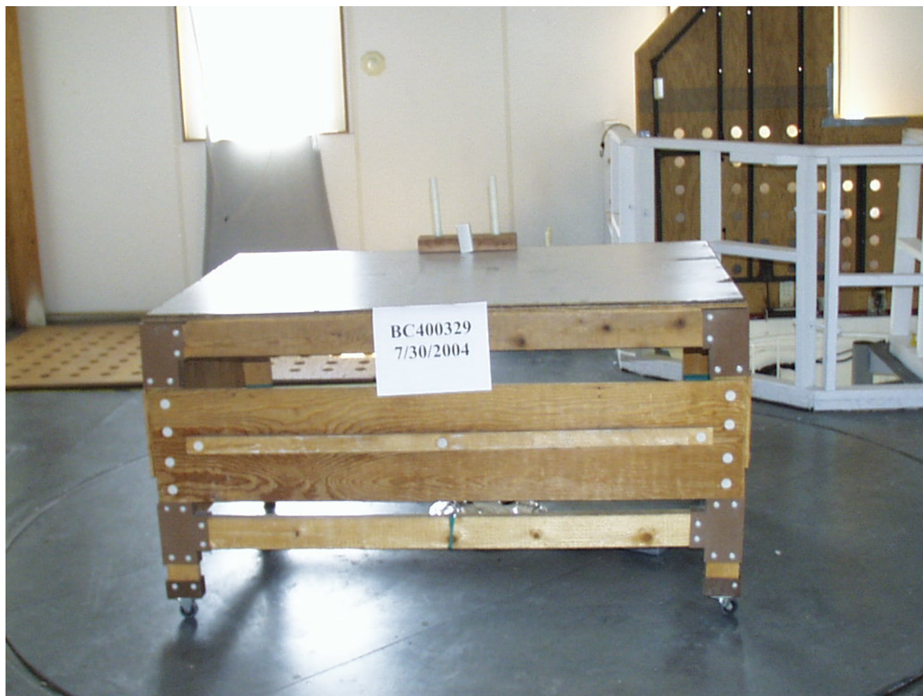
Test-setup photo(s): Radiated Unintentional Emissions
