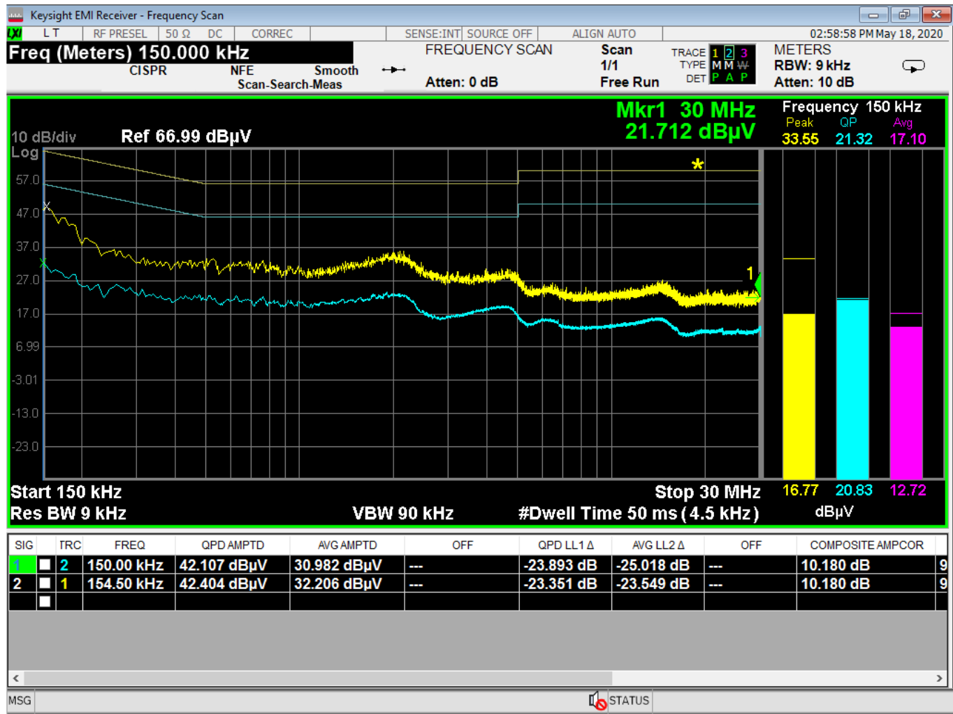
Figure 30 - Conducted Emissions Plot, Neutral
