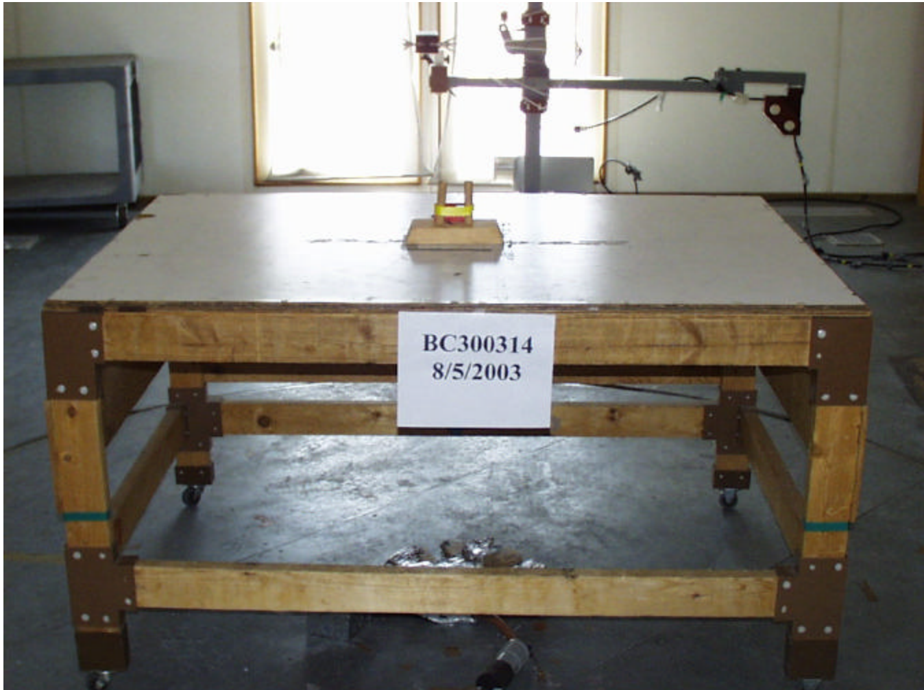
Test-setup photo(s): Radiated Emissions
