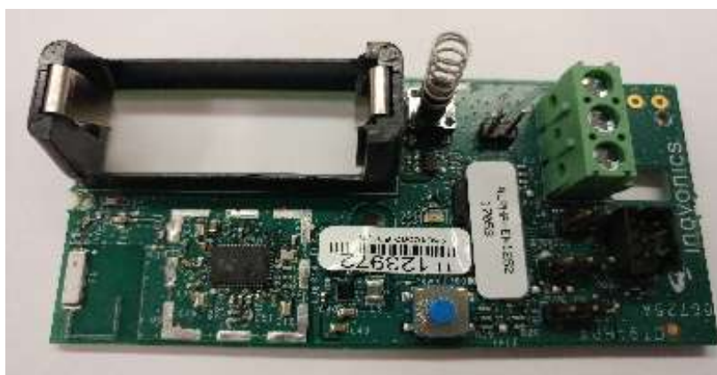
Picture 2 - EN1252 Top View Shield Can Removed
