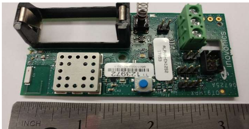
Picture 2 - EN1252 Top View Shield Can Removed
