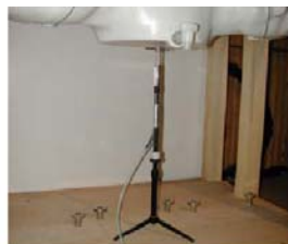
Figure 9.1 Dipole Verification Test Setup Diagram & Photo
