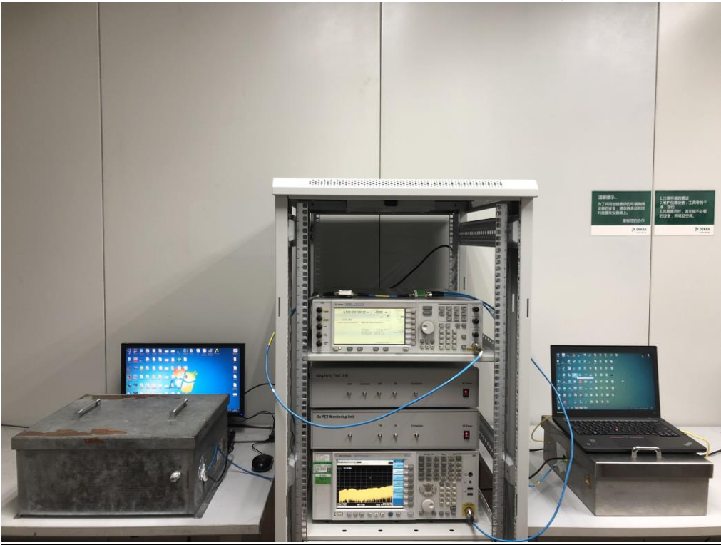
DFS Set-up Photo: Slave and Spectrum Analyzer
