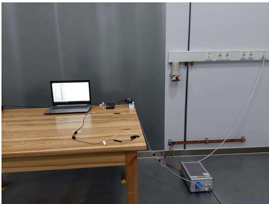
Fig. 3 Power line conducted emission setup photo
