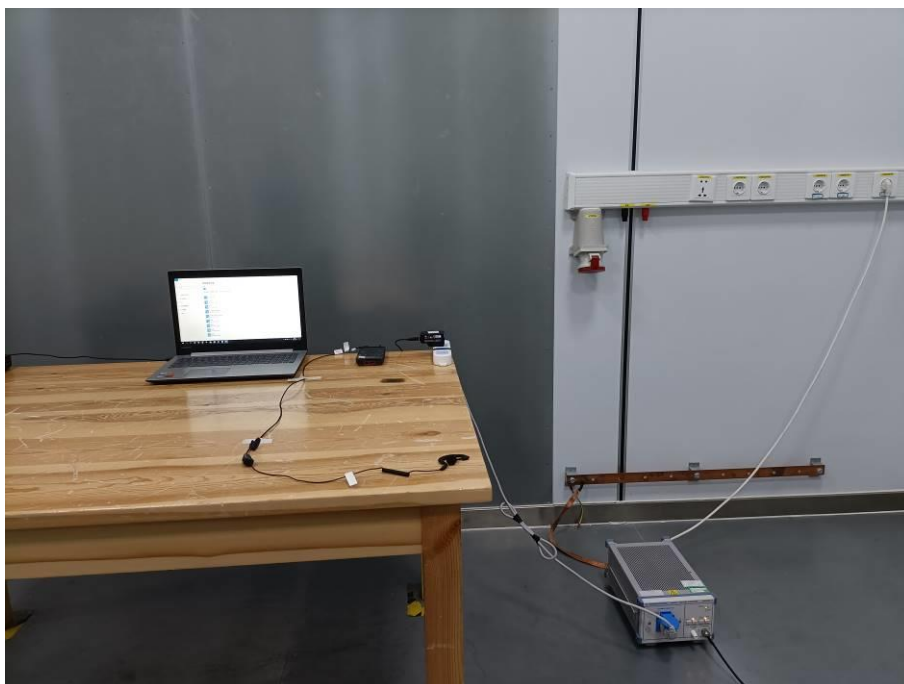
Fig. 3 Power line conducted emission setup photo
