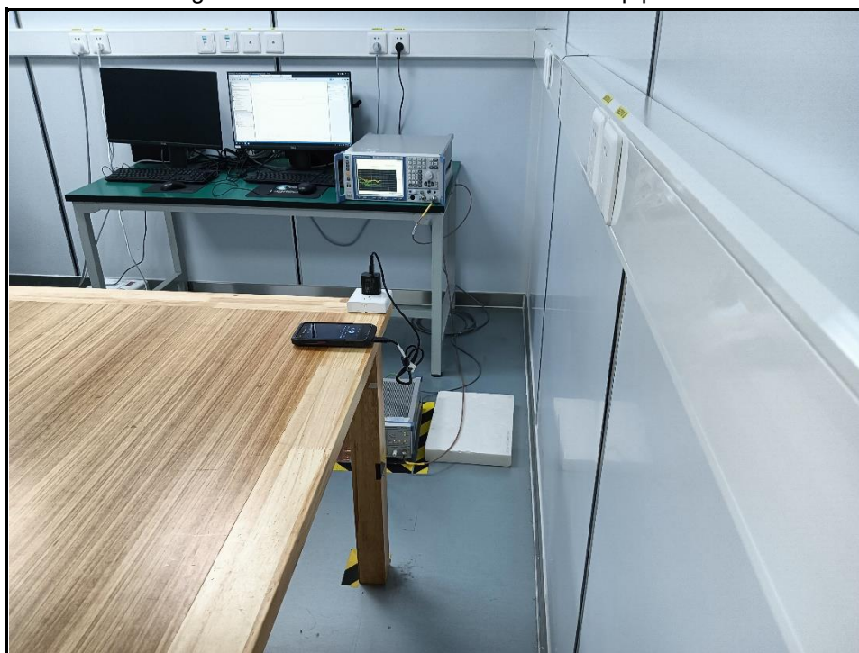
Fig. 4 Power line conducted emission setup photo
