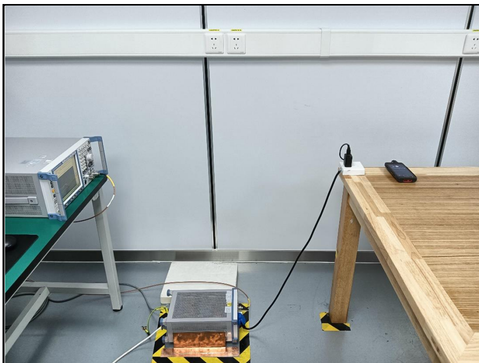
Fig. 3 Power line conducted emission setup photo
