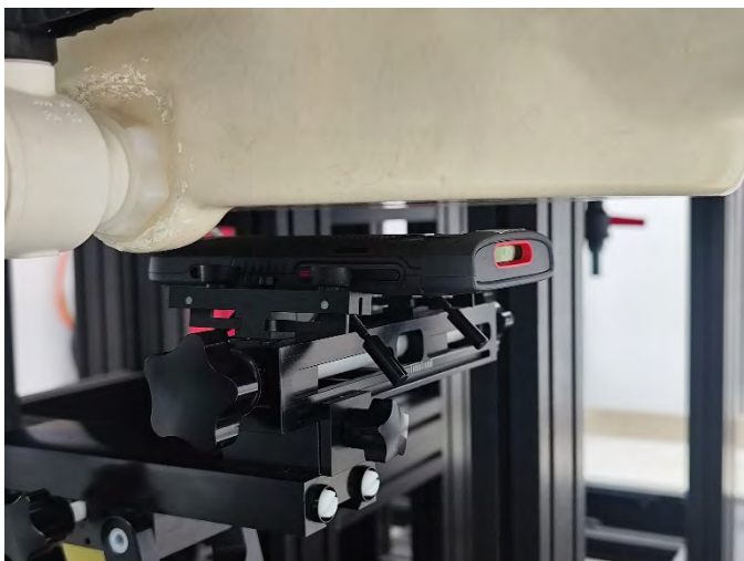
Rear Face of EUT with 1.5 cm Gap (Body Mode)
