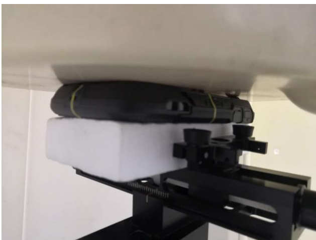
Rear Face, Test Separation 0 mm
