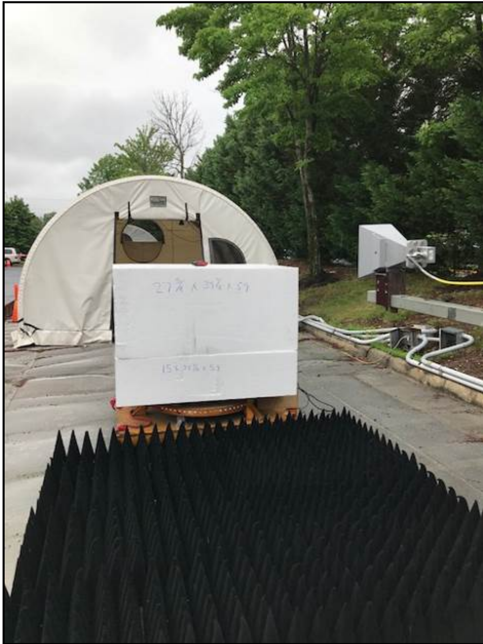
Photograph 1: Radiated Emissions Testing – Front View (Above 1 GHz)
