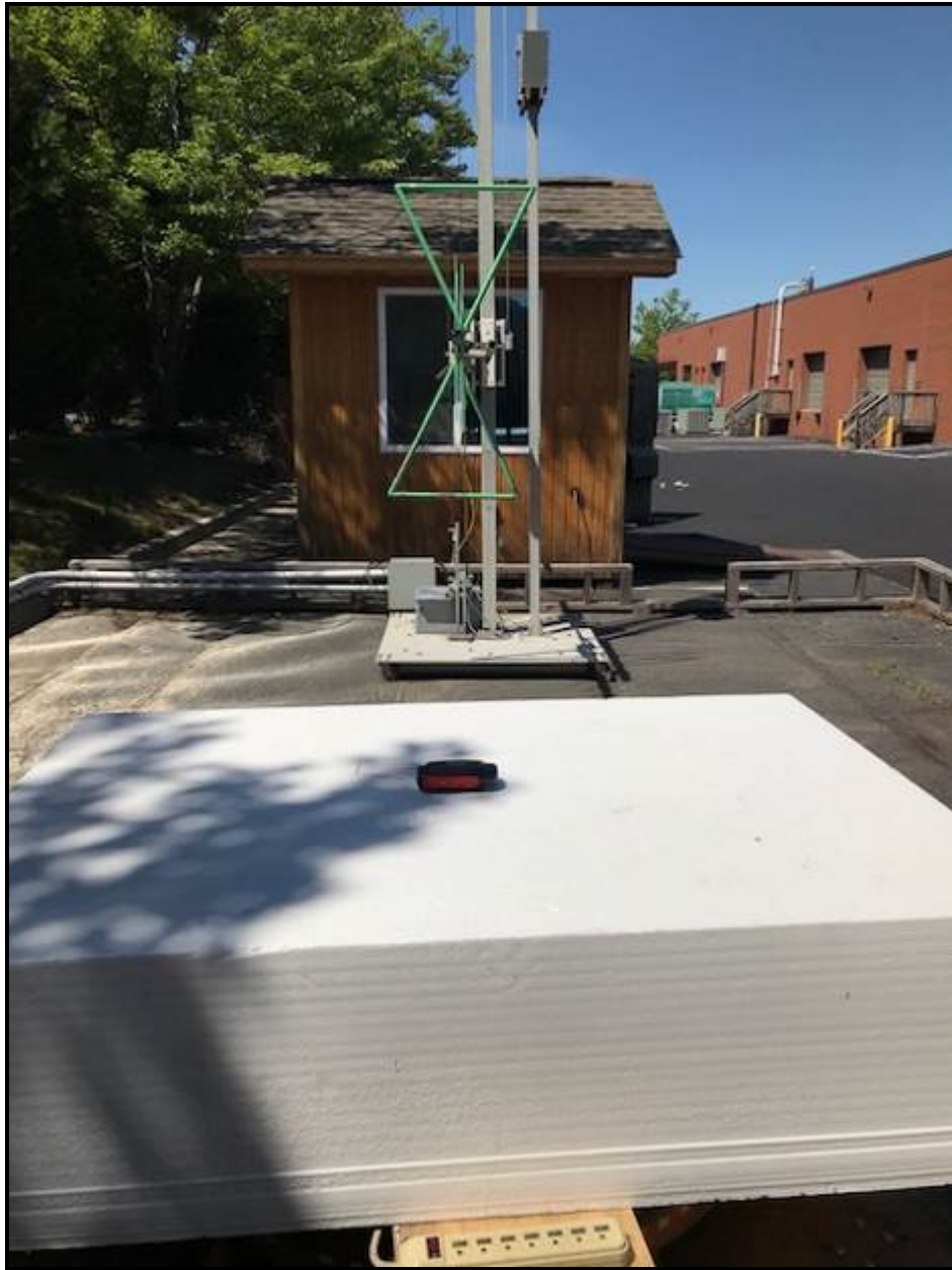
Photograph 4: Radiated Emissions Testing – Back View (Below 1 GHz)
