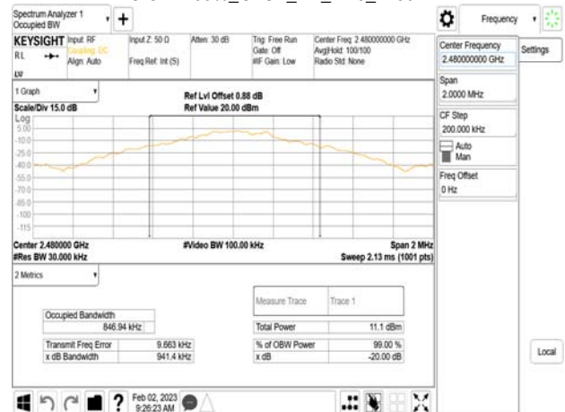
IC OBW 99%_GFSK_1M_DH5_2480MHz
