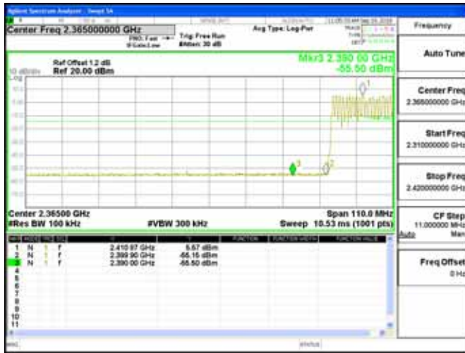
Hopping Band Edge_GFSK_1M_DH5_2480MHz
