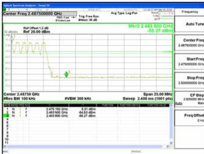
Hopping Band Edge_GFSK_1M_DH5_2480MHz
