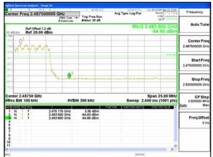
Hopping Band Edge_8DPSK_3M_DH5_2480MHz
