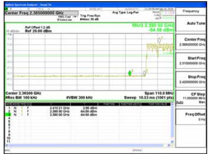
Hopping Band Edge_8DPSK_3M_DH5_2480MHz
