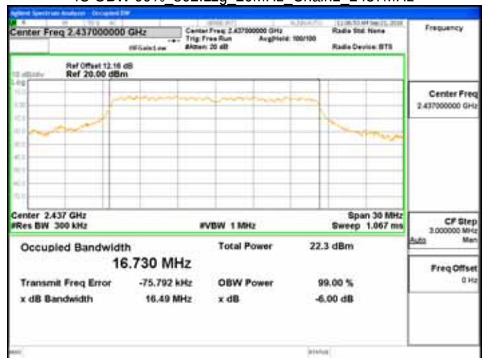
IC OBW 99% 802.11g_20MHz_Chain1_2462MHz
