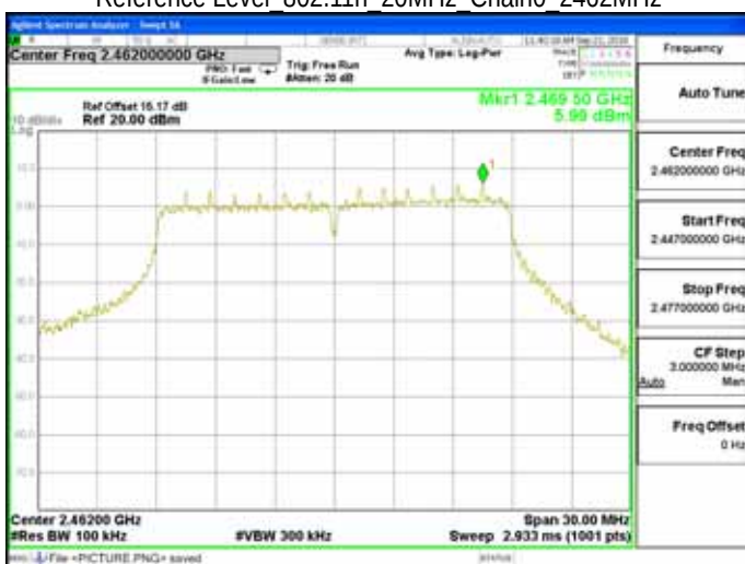
Reference Level 802.11n 20MHz Chain0 2462MHz
