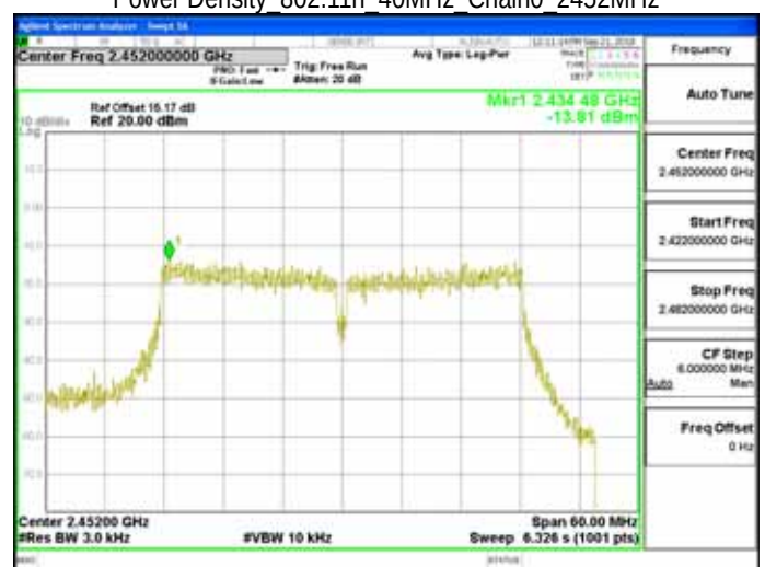
Power Density 802.11n 40MHz Chain0 2452MHz
