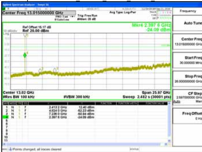
Spurious Emission 802.11b 20MHz Chain0 2437MHz
