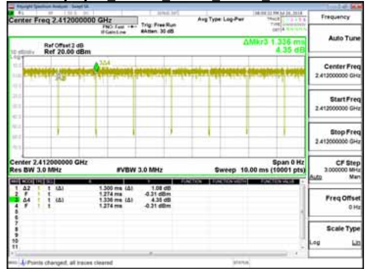
Duty Cycle 802.11n 40MHz Chain0 2422MHz
