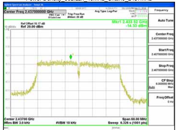
Power Density 802.11n 40MHz Chain0 2452MHz
