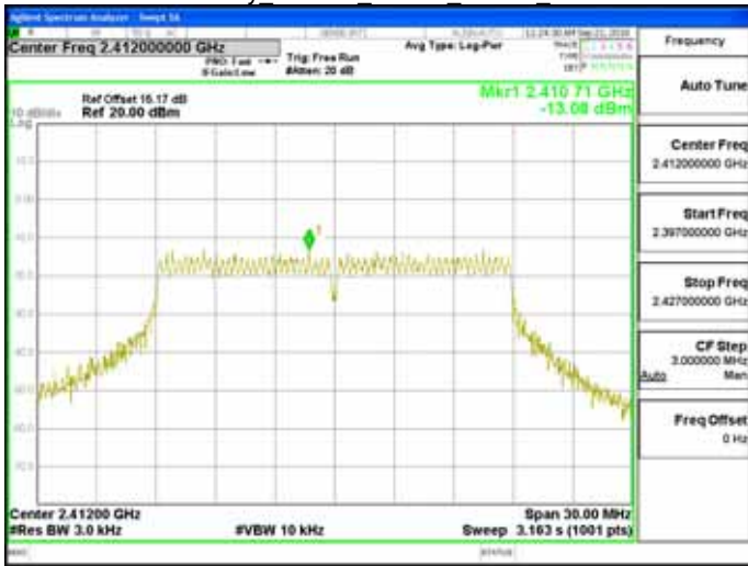
Power Density 802.11n 20MHz Chain0 2437MHz
