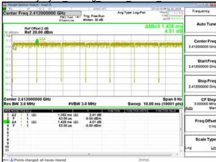
Duty Cycle 802.11g 20MHz Chain0 2412MHz
