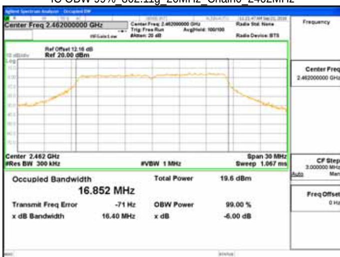
IC OBW 99% 802.11g_20MHz_Chain0_2462MHz
