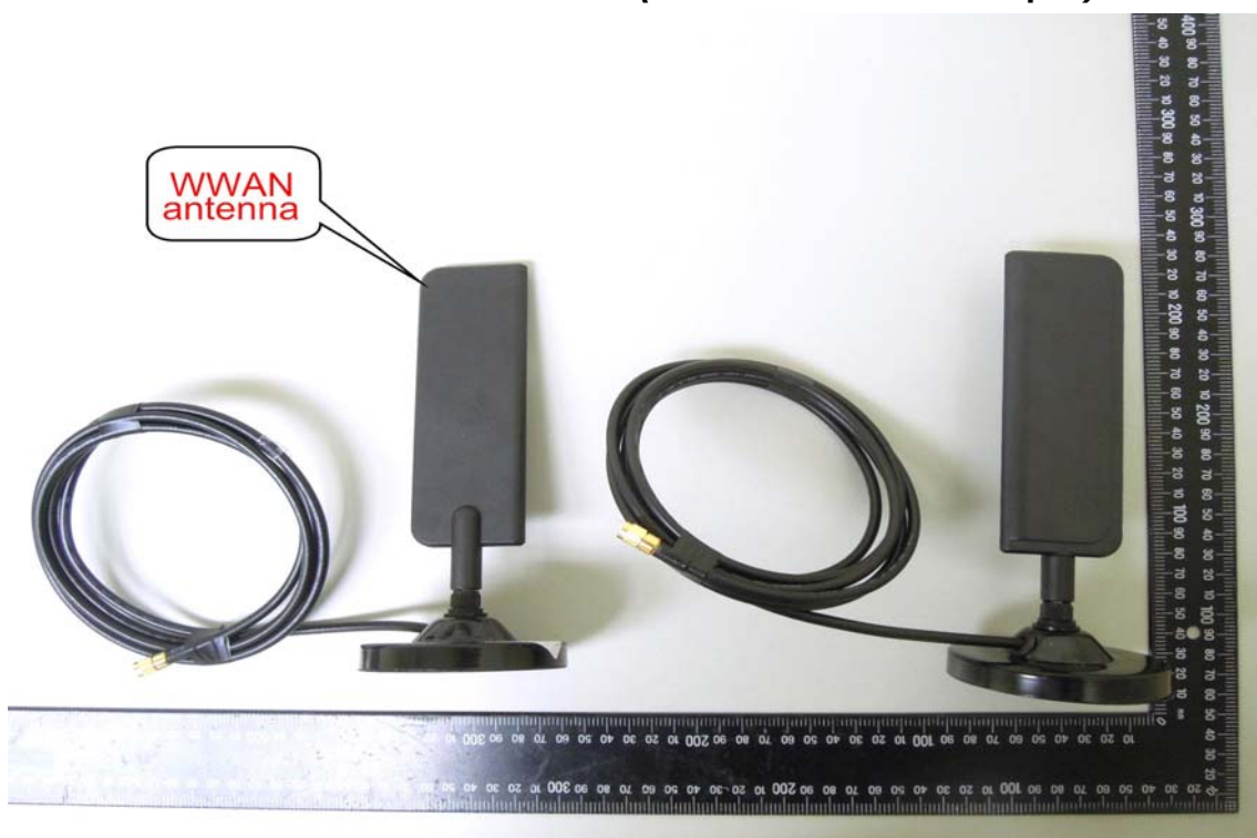
WWAN External Antenna-4 (Part No.: TG.30.8111 Apex)
