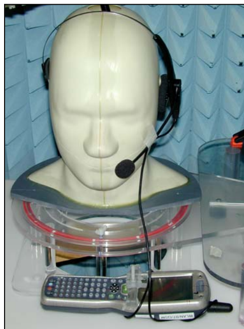
Figure 44. A Positional photograph of D9500 Device Fitted with Normal Battery positioned For Headset testing LH Cheek.
