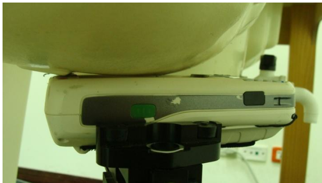
Right Cheek (DUT with KeyPad 31)
