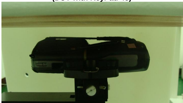
Bottom of the DUT with Phantom 1.5 cm Gap (DUT with KeyPad 45)
