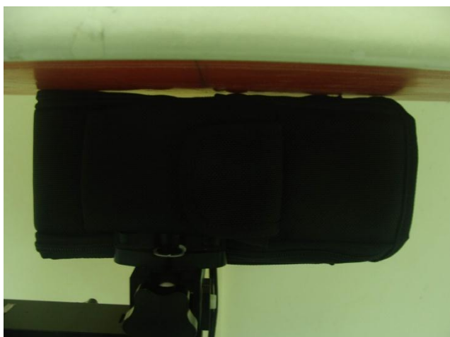
Left side of the DUT with Holster with Phantom 0 cm Gap
